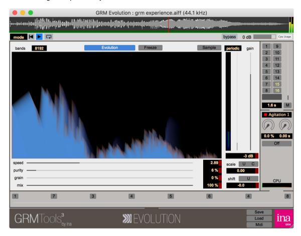
In this version, the processing window includes at the top a strip to control the reading and writing of sound files.
