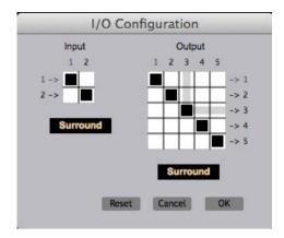
In this example, the processing is configured as a stereo input and output on 5 channels. The sequencer track channels (n-> or -> n) correspond to the rows of the matrices. The input and output channels of the processing correspond to the columns of the matrices. To direct a process output channel to a channel of the output track (or an input track channel to a process input channel), click in the corresponding box of the matrix.
